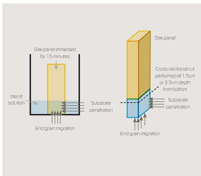
Figure 4: 1.5 cm depth cross-section of oak panels after 15 minutes dip.
