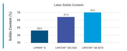
Higher solids content can support the drying property and reduce shrinkage after drying.
